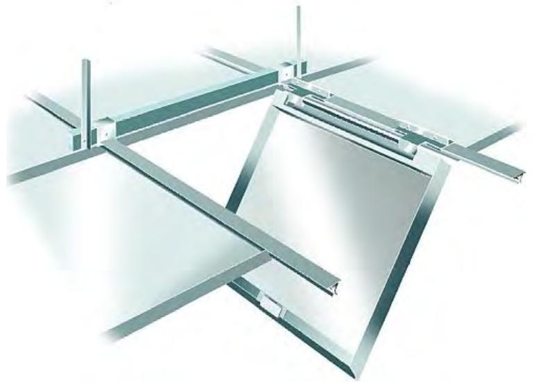
The panels are manufactured with reinforced frames that provides rigidity to the panel whilst permitting the panel to hinge down for access to the ceiling plenum. Access panels are fitted with locking devices to retain the panel in the ceiling which can be operated with a square shanked key (Budget Locks); in sensitive areas such as police stations or prisons the locks can be key operated (Yale Type).
