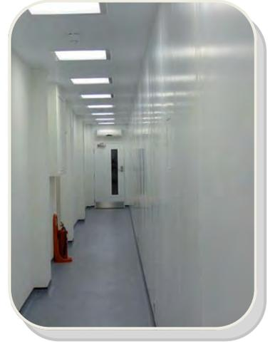
The finish is white powder coated, and the panels are supplied 1200 mm wide with a single line joint. Panel depth will range from 100 mm to 250 mm depending upon span and other requirements. Perimeter trims are also included.
